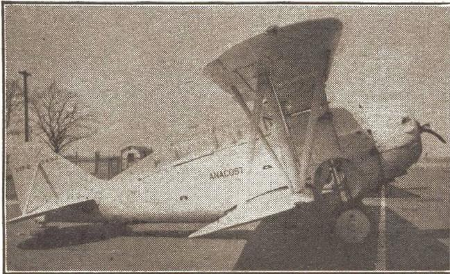
THE Navy is going in strong for the Grumman! This is the new XF2F-1 two-place shipboard fighter. It mounts a Twin-Wasp, which gives the craft considerable more speed than the original model which employed a 710-h.p. "Cyclone" and had a top of 197 m.p.h.
